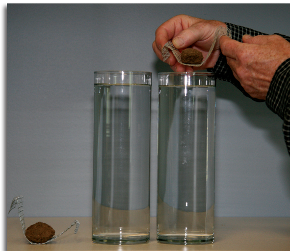
The slake test demonstrates how soil glues hold soil particles together to resist disintegration into individual particles.
