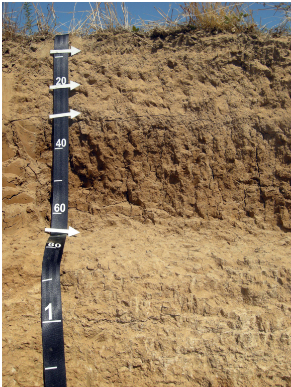
Fig. 2. Soil Profile of a San Joaquin soil illustrating horizons and horizon boundaries. Credit: USDA-NRCS.
