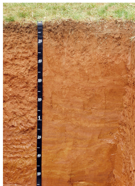
Fig. 1. Soil profile of a Sunnyside soil formed in loamy fluviomarine sediments. Credit: USDA-NRCS
