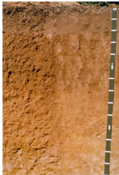
Fig. 1. Soil profile of a Sassafras soil formed in sandy marine sediments. Credit: USDA-NRCS
