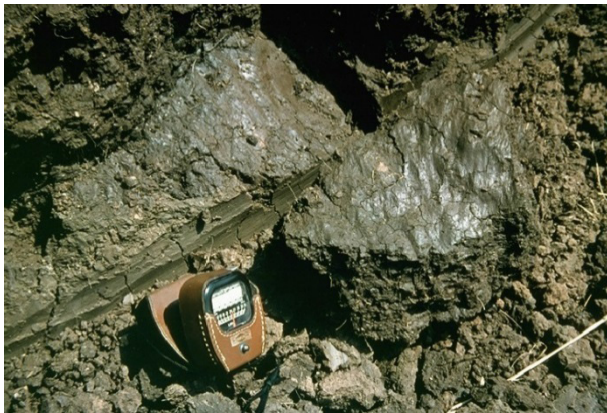
Fig. 4 Slickensides are polished, grooved surfaces caused by the surfaces sliding against each other during shrinking and swelling of the soil. Credit: Soil Science Society of America
