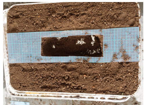
E) “Rain garden” construction. Potting mix was used to replace soil removed from the center of the pan. The rain garden helps to absorb water and slow runoff. Runoff volume was reduced by 23% compared to the impervious surface without the rain garden. Real rain gardens could function as wetlands, contain plants to use collected water, or simply retain water for slower discharge.
